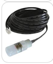
AVTECH's Digital Fluid Temperature Sensor monitors the temperature of fluids in refrigerated and other environments using a unique sensor housing. The temperature sensor is sealed in a tube filled with propylene glycol, a nonconductive clear liquid with a low freezing/high boiling point. The sensor returns the readings of the propylene glycol so that you may measure the consistent temperature held by the fluid rather than the ups and downs of the air moving around it.
