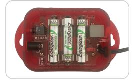
Test the unit regularly to make sure it is fully operational. To test the batteries, unplug the MUPS from power—making sure the Battery Backup Button is pushed in—and check that the Status LED is fully lit red. (Dim red may indicate the batteries are partially charged; an unlit Status LED indicates there's no charge.)
