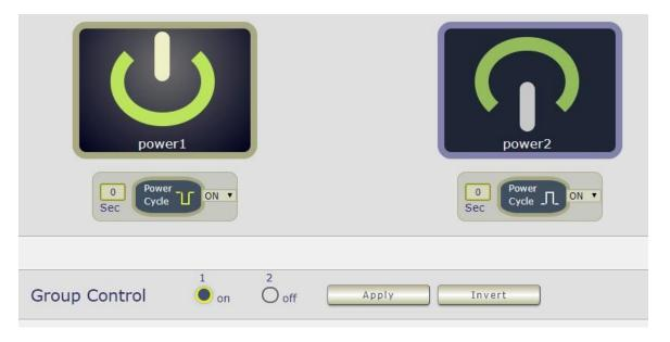
The following 3 pictures shows that after press the power cycle with 5 seconds setting , the outlet "Power1" will turn off for 5 seconds , then turn ON later . The power cycle action will execute after press the "Power Cycle" button .
