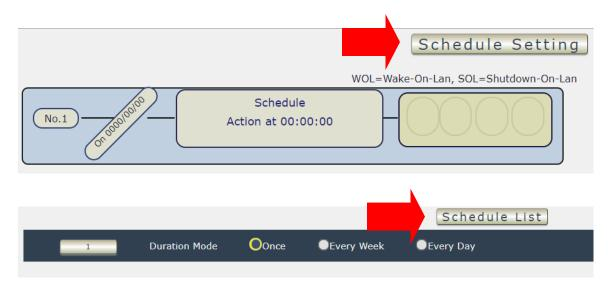
The schedule allows you to control the power outlet or turn ON / OFF/ RESET at assigned time
